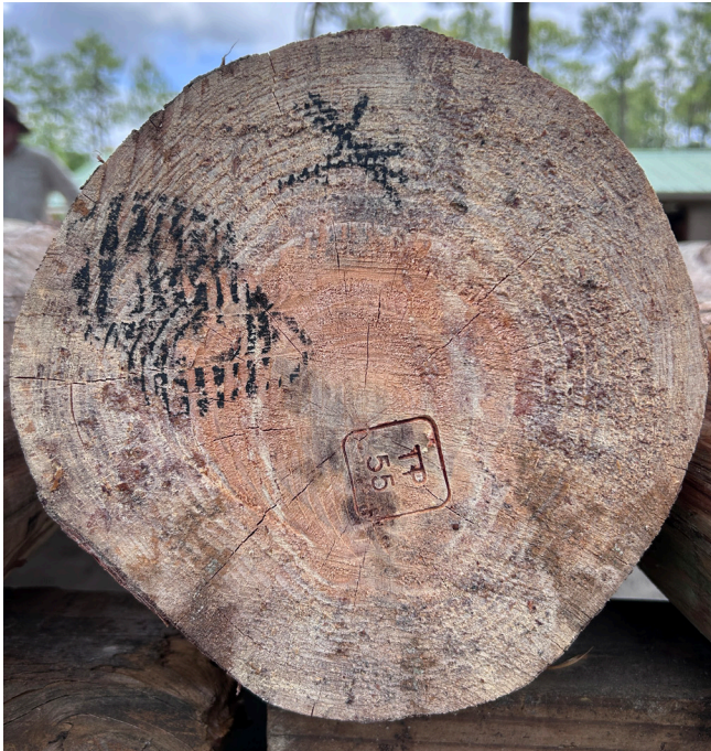
Figure 4. An example SYP log after review and certification by a third-party log grader. For the MASS Haptic pavilion, the TP 55 stamp remained visible on all logs through the final installation of the structure. Image Credit: Atelier Mey
